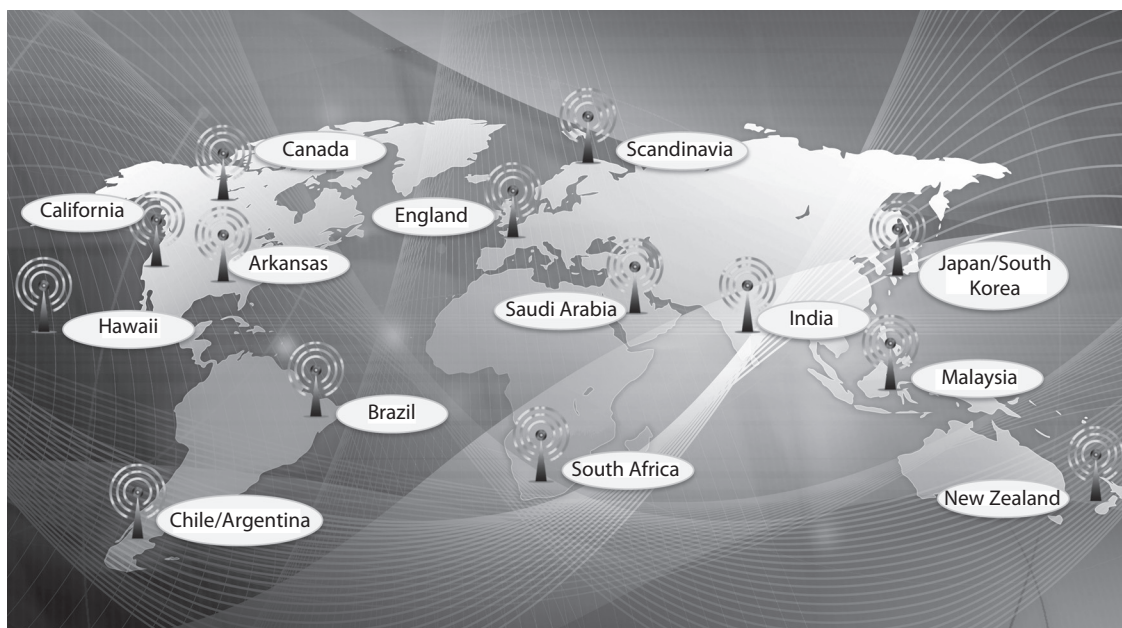
FIGURE 37.1 Proposed locations for the global network of monitoring sites. These sites are specifically designed to measure the magnetic resonances in the earth-ionosphere cavity, resonances that are generated by the vibrations of the earth's geomagnetic field lines, and ultra-low frequencies that occur in the earth's magnetic field.
